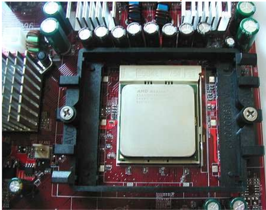
The Athlon 64 retention mechanism (here on the MSI K8T Neo) is efficient and user-friendly
