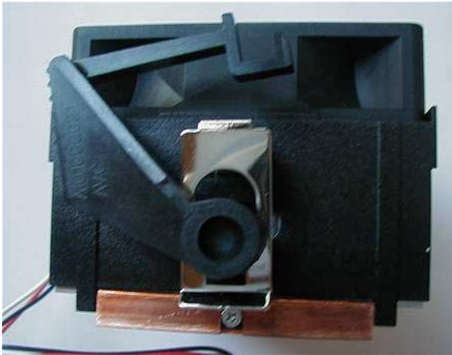
Typical heatsink solution for the Athlon 64: massive heatsink but slow 3000 rpm fan. Note the special safety hook on the lever
