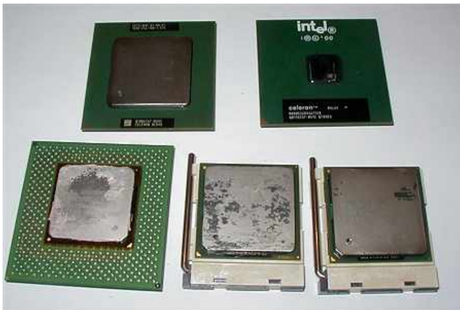
The Intel Family! Top: left Celeron Tualatin, right Celeron Coppermine Bottom: Pentium 4 Willamette 423, Pentium 4 Willamette 478 pin, Pentium 4 Northwood
